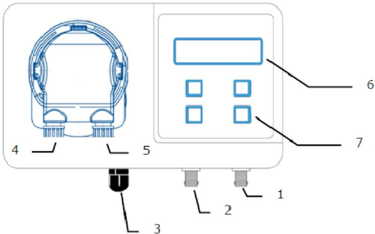
1. BNC socket for container level switch
